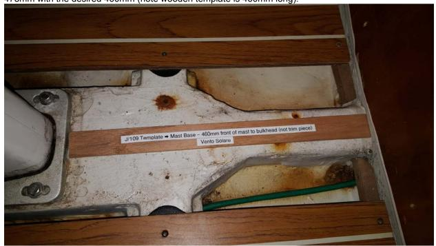
This is mast base position with it all the way forward. Actual distance is 466mm (6mm short of target 460mm) and unless the holes are re-drilled, the mast shoe will not slide any further forward.
