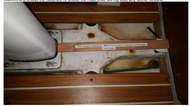
The floorboards installed with the trim pieces off. The gap at the aft end is barely covered by the trim
