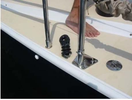
Rather than tying up the block this boat used one of the Harken rubber stand ups. This fitting also works well on the bow sprit block if you use one.
