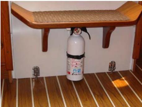
This is a good place for a fire extinguisher. When you remove the stairs the extinguisher helps hold the stairs from sliding out when you prop the stairs against something when accessing the engine area.
