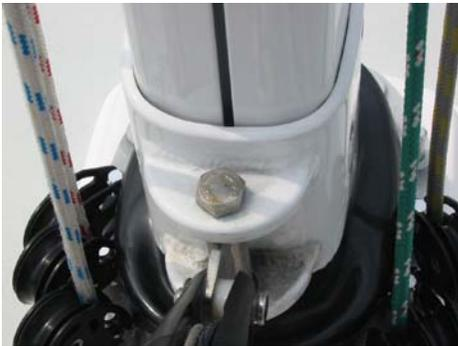
This is the newer vang fitting. You can also see the nylon washer between the vang and the stainless fitting the vang attaches to in order to prevent the vang from twisting. This is also recommended for the vang-to-boom attachment as well.
