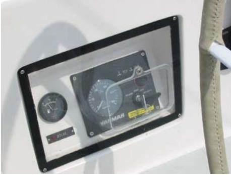
This panel has been removed and the edge painted black on the back and then reinstalled. This is a cleaner look and hides the gasket material that tends to deteriorate with sunlight.
