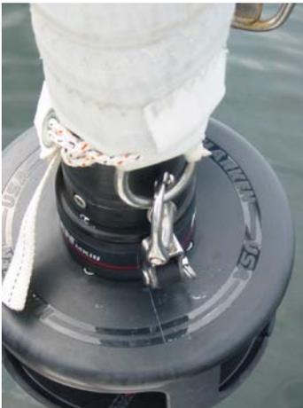
Wichard Snap Shackles were seen on 90% of the boats for the tack of the jib and the head of the jib to prevent the bowman from losing the shackles when removing the sail after racing.
