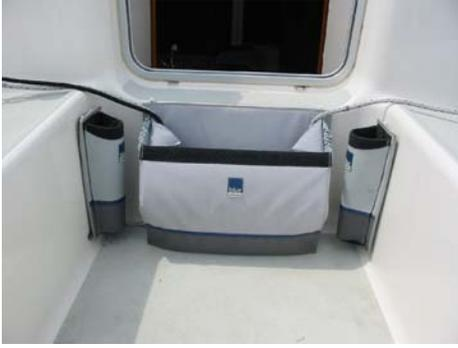
Blue Performance line bag and winch handle holders. The nice thing about these is that they weather better and can be removed easily for winter storage. This boat has the large bag and we have found that the Medium bag works best in this location so that the winch holders can also mount to the front face of the cockpit.
