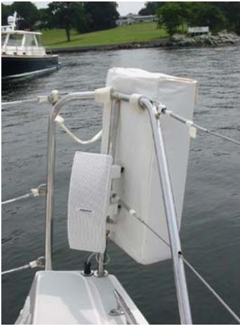
Speaker option: Even the bowman can hear the stereo clearly when mounted here. The captive removable clamps are nice. The potential problem point is corrosion at the plug.
