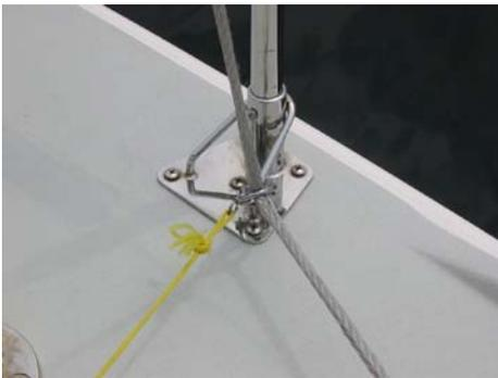
Method two is to use a Wichard snap shackle with a trigger line led to the opposite handrail for easy deployment of the halyard from the windward rail.
