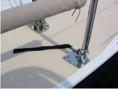
This is one of two methods used to secure the spinnaker halyard to the rail. This boat was using Velcro to hold the halyard.
