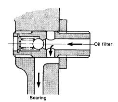
When the pressure is lower that the regulated pessure
