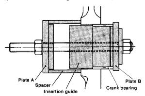
until it touches the cylinder block or bearing housing, using the puller/extractor as a guide, as shown in the figure.
