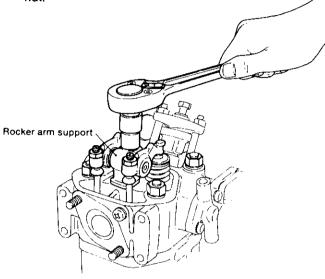
CAUTION: 1. Loosen the valve head clearance adjusting screw in advance.
