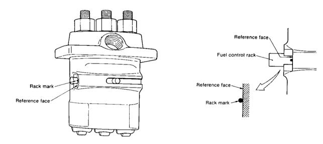
NOTE: When the engine is stopped, the control rack will automatically stay at the position which allows the maximum fuel injection volume.
