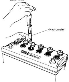
2) Take the specific gravity reading at the top of the scale of the hydrometer.
