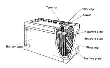
The battery utilizes chemical action to convert chemical energy to electrical energy. This engine uses a lead acid battery which stores a fixed amount of power that can be used when required. After use, the battery can be recharged and used again.
