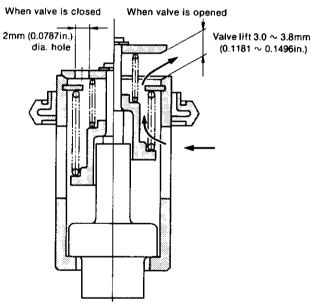
A wax-pellet type thermostat is used for this engine. The "wax-pellet" type is the description given to a quantity of wax in the shape of a small pellet. When the temperature of the cooling water rises, the wax melts and its volume expands. The valve is opened or closed by this variation of volume.
