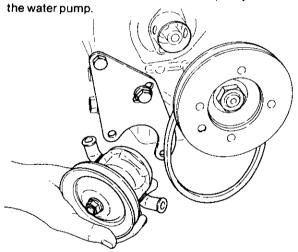
(2) Tighten while adjusting the V-belt tension
