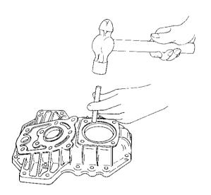
9-4 Insert the center bush and location pin to the clutch case end holes.
