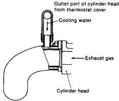
As shown in the figure, the construction for models 1GM10(C) and 2GM20(F)(C) is such that there is no exhaust manifold and the mixing elbow is fitted to the exhaust gas outlet port. A double construction technique has been adopted for the mixing elbow; as the exhaust gas passes through it the cooling water passes round the outside to cool the exhaust gas and then the gas and water mix close to the outlet port.
