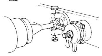
NOTE: Attach the bushing to the piston pin so that the pin, coated with engine oil can be pushed into position with your thumb.
