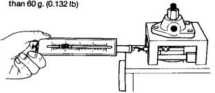
NOTE: If the sliding resistance is unsatisfactory, disassemble, inspect and repair the fuel control rack.
