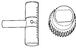
(3) If the control rack does not move smoothly when a force of within 60g is applied, replace the rack and pinion assembly.
