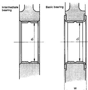
diameter. As the flange wears away the side gap of the crankshaft increases.
