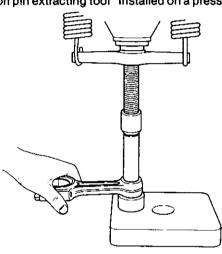
NOTE: Force the piston pin bushing into position so that its oil hole coincides with the hole on the small end of the connecting rod.
