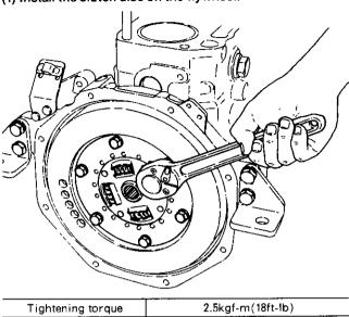
(2) Align the disc and input shaft spline, and install the clutch assembly on the mounting flange.
