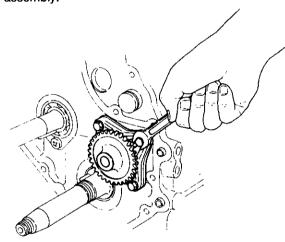
NOTE: Do not separate the lubricating pump gear from the rotor shaft. If removed, it cannot be used again. When any part is unusable, replace it as a complete assembly.
