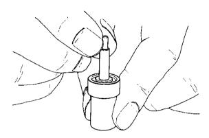
(4) The nozzle must be fitted on the nozzle holder with the nozzle spring retainer loosened.
