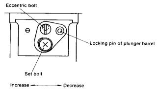
By loosening the set bolt and turning the eccentric bolt clockwise, the position of the pin moves to the left to increase the injection volume, and by turning the eccentric bolt counterclockwise, the pin moves to the right to decrease the injection volume.
