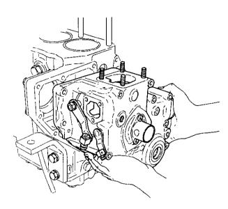
(2) Remove the lubricating oil pump driving gear and pump assembly.
