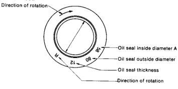
(4) Insert the oil seal with a press. However, when unavoidable, the seal may be installed by tapping the entire periphery of the seal with a hammer, using a block. In this case, be careful that the oil seal is not tilted. Never tap the oil seal directly.
