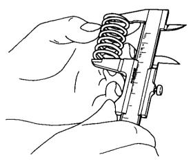
Also, measure the tension of the spring with a spring tester. If the tension is below the prescribed limit, replace the spring.
