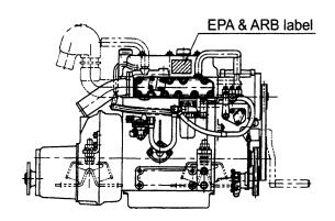
\*3GM30F(C)(V): attached to the top of the fresh water cooler.
