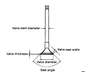
mm (in.) 1GM10(C) 2GM20(F)(C) 3GM30(F)(C) 3HM35(F)(C)  $\phi$ 32 (1.2598)  $\phi$ 32 (1.2598) Exhaust valve diameter  $\phi$ 26 (1.0236)  $\phi$ 27 (1.0630)
