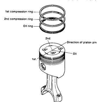
(4) Insert the piston connecting rod assembly so that the side of the connecting rod large end with the identification number is on the exhaust side. Install the piston rings with a piston ring inserter.
