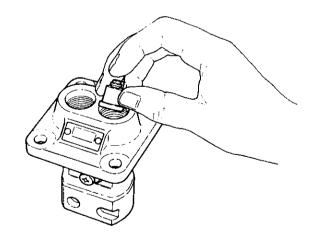
NOTE: If the delivery valve tip projects noticeably above the top of the main unit of the pump, the plunger barrel has been installed incorrectly, and must be re-attached.
