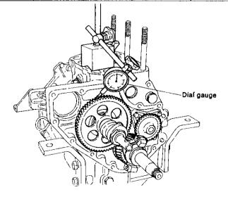
(2) Insert a piece of quality solder between the gears to be measured and turn the gears. The backlash can be measured by measuring the thickness of the crushed part of the solder.
