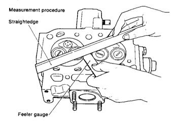
(4) The thickness of the largest feeler gauge that can be inserted is the amount of distortion.
