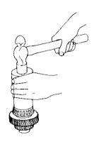
9-3 Fit the bearing outer races in the V-drive cases A and B.
