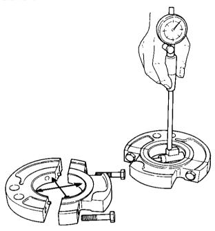
mm (in.) 2GM20(F)(C), 3GM30(F)(C) 3HM35(F)(C) Maintenance standard Wear limit Maintenance standard Wear limit Ø44.0 (1.7323) Ø44.12 (1.7370) Ø47.0 (1.8504) Ø47.12 (1.8551) Gear case side intermediate bearing inside diameter D Ø47.12 (1.8551) Ø44.0 (1.7323) Ø44.12 (1.7370) Ø47.0 (1.8504) Flywheel side intermediate bearing inside diameter D. 25-0.09 30-0.09 29.63 2463 Width of intermediate bearing (Flywheel side) (1.665)(0.9697) $(1.1744 \sim 1.1776)$  $(0.9776 \sim 0.9807)$
