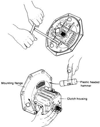
(8) Withdraw the output shaft assembly.
