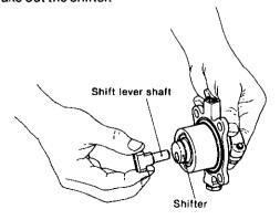
(4) Withdraw the shift lever shaft.
