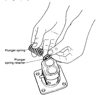
NOTE: The plunger spring retainer should face the underside the pump.
