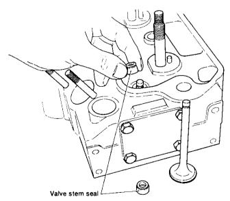
A valve stem seal is assembled at the top of the valve guide and the valve stem chamber oil is sucked into the combustion chamber through the valve guide (oil down) to prevent an increase in oil consumption.
