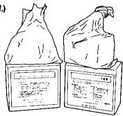
Cooling passage cleaner is made by adding one part "Unicon 146" to about 16 parts water (specific gravity ratio). To use, drain the water from the cooling system, fill the system with cleaner, allowing it to stand overnight (10  $\sim$  15 hours). Then drain out the cleaner, fill the system with water, and operate the engine for at least one hour.
