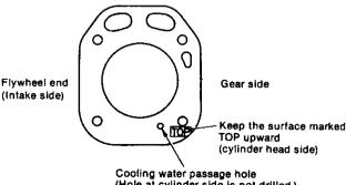
Cooling water passage hole (Hole at cylinder side is not drilled.)
