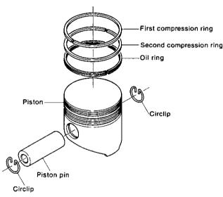
A complete set of piston rings consists of two compression rings and one oil ring.
