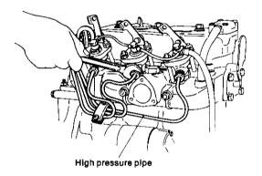
NOTE: Use the special high pressure pipe for a fresh watercooled engine. The shape and dimensions are different from those for a sea water-cooled engine.
