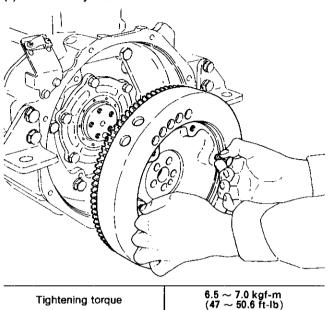
NOTE: After tightening, check the end run-out
