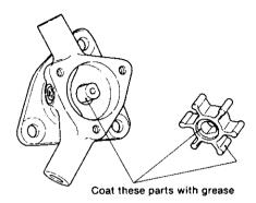
(2) Be sure that the direction of curving of the impeller is correct.
