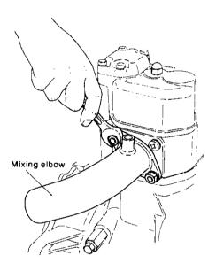
Check for carbon build-up and for corrosion inside the pipe, and repair or replace the pipe if faulty.
