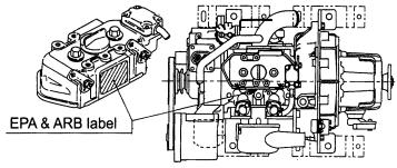
\*3GM30(C)(V): attached to the exhaust side of the rocker arm cover.
