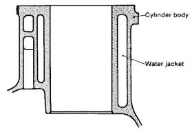
The cylinder block is a high-quality cast iron casting, with integral cylinders and deep skirt crankcase construction. As a result of stress analyses, the shape and thickness of each part has been optimized, and special ribs employed which not only increase the strength and rigidity of the block, but also reduce noise.
