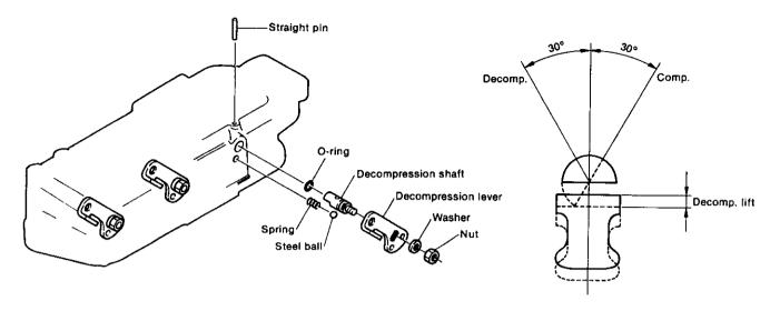
With this engine, there is no need to adjust the decompression lift.
