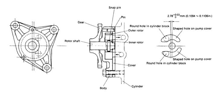
2-1.3 Specifications of lubrication oil pump
