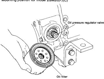
When the pressure is lower than the regulated pressure
