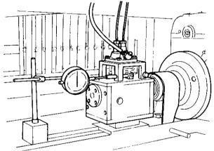
(3) Run the pump tester at low speed, loosen the air bleeder screw, and bleed the air from the injection pump.
