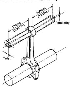
Pass a test bar through the large end and small end holes of the connecting rod, place the bars on a V-block on a stool and center the large end test bar. Then set the sensor of a dial indicator against the small end test bar and measure twist and parallelity. When the measured value exceeds the wear limit, replace the connecting rod. Twisting and poor parallelity will cause uneven contact of the piston and bushing and shifting of the piston rings, resulting in compression leakage.
