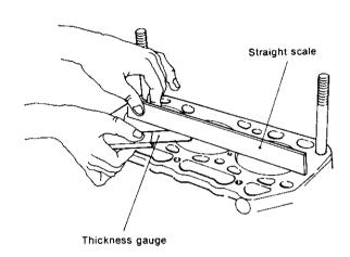
Measurement is to be carried out on the 4 sides and 2 diagonal lines as shown in the figure, and the largest value of clearance for each measurement is to be taken as the amount of distortion.
