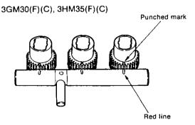
NOTE: After attaching the fuel control pinjon to the main unit, check its meshing by moving the fuel control rack.
