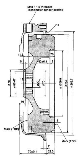
NOTE: Material of flywheel housing. Sail-drive type: Cast iron Marine gearbox type: Aluminum alloy
