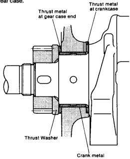
On models 2GM20(F)(C) and 3GM30(F)(C), the value of the side gap is the difference between the width of the basic bearing metal and the width of the journal. The basic bearing for model 2GM20(F)(C) is the intermediate bearing, and for models 3GM30(F)(C) and 3HM35(F)(C) it is the intermediate bearing at the flywheel end.
