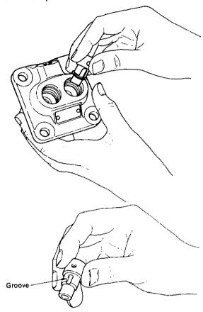
(3) Install the No.1 delivery valve, delivery valve seat and packing.
