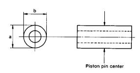
Maximum wear measured in (a) (b) directions at central position marked\*
