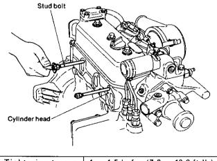
Tightening torque  $1 \sim 1.5 \text{ kgf-m}(7.3 \sim 10.9 \text{ ft-lb})$
