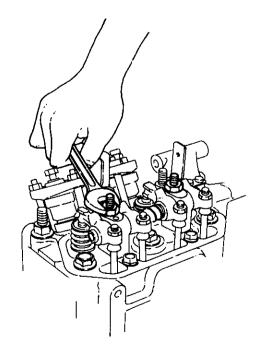
3) Remove the rocker arm retainer, and pull the rocker arm from the rocker arm support.
