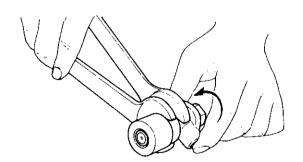
(5) When installing the injection nozzle on the cylinder head, tighten the nozzle holder nuts alternately, being careful to tighten them evenly.
