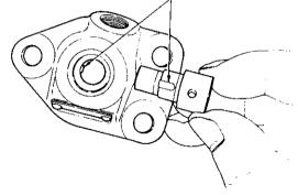
(2) Attach the delivery valve seat and the delivery valve to the main unit.
