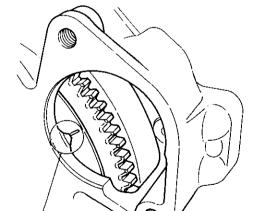
With respect to models 1GM10(C), 2GM20(F)(C) and 3GM30(F)(C) only, a projection which serves as the matching mark is provided in the cast hole of the clutch housing.
