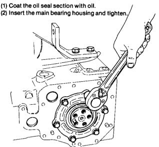
(3) Check that the crankshaft rotates smoothly.
