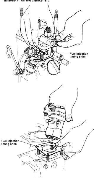
(8) Finally, turn the crankshaft slowly and confirm that it turns easily. If it is stiff or does not rotate, the plunger head gap is too small.
