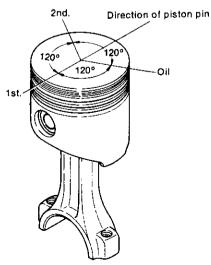
5) Since the oil ring is equipped with a coil expander, attach it to the piston so that the joint of the ring is opposite the gap of the coil expander.
