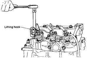
NOTE: Use the special lifting hook for the fresh water-cooled engine.
