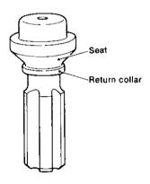
(2) Raise the delivery valve and put a finger over the hole on the valve seat bottom. Let go of the delivery valve. If it sinks quickly and stops at the position where the suckback collar closes the valve seat hole, the delivery valve may be considered normal. If this is not the case, replace the delivery valve as a set.
