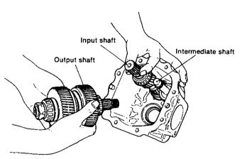
(9) Take out the intermediate shaft and input shaft. When taking out the intermediate shaft, place a bolt or spacer on the shaft hole of the case, and drive the shaft out by tapping it lightly.
