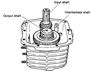
(10) Remove the output shaft, intermediate shaft, and input shaft from the case, in that order.
