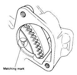
With respect to models 1GM10(C), 2GM20(F)(C) and 3GM30 .(F)(C) only, a projection which serves as the matching mark is provided in the cast hole of the clutch housing.
