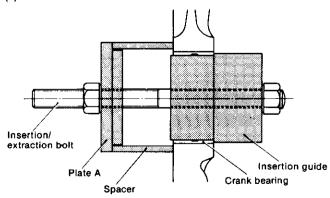
Assemble the spacer and plate A as shown in the figure, place the puller/extractor against the bearing from the opposite end and pull the bearing by tightening the nut of the special tool. Remove the oil seal before pulling the bearing pressed against the bearing housing.
