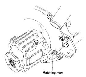
NOTE: Set to the position at which the valve rocker arm shaft does not move even when the crankshaft is turned to the left and right, centered around the matching mark.
