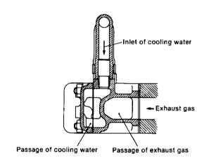
The construction of the exhaust manifold is shown in the figure, and a water chamber is formed between the exhaust manifold and the cover to cool the exhaust gas. The construction of the mixing elbow is the same for models 1GM10(C) and 2GM20(F)(C)
