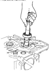
NOTE: Be careful not to damage the groove in the end of the shaft.
