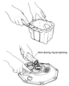
(9) Insert the input shaft and output shaft into the shaft holes of the mounting flange, assemble the mounting flange on the case body, and tighten the bolt.
