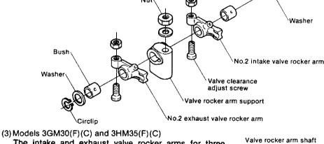
The intake and exhaust valve rocker arms for three cylinders are fitted to a valve rocker arm shaft at both sides of the spring. The same intake and exhaust valve rocker arms, valve rocker arm support, spring and valve clearance adjusting screw are used for models 3GM30 (F)(C) and 3HM35(F)(C).
