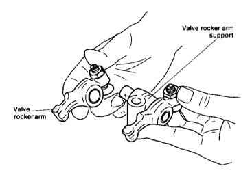
NOTE: A retainer is not used for the valve rocker arm on model 1GM10(C) and is kept free, therefore the rocker arm can be removed directly.
