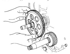
(3) Tighten the camshaft end nut.
