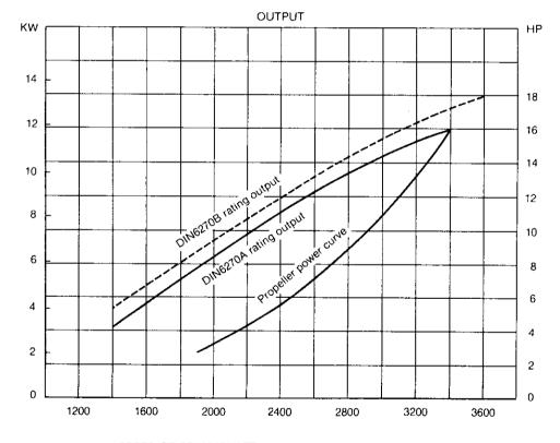
SPEED OF CRANKSHAFT: rpm
