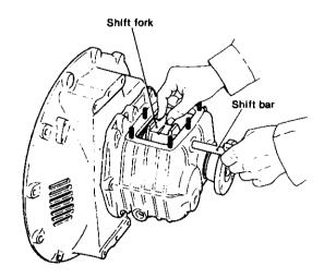
(2) Coat the threaded part of the shift bar plug with a nondry packing agent and secure it to the case with a hexagonal bar spanner (width across flats: 8mm (0.3150in.).
