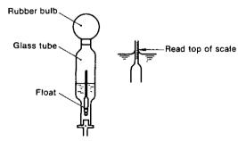
3) The battery is fully charged if the specific gravity is 1.260 at an electrolyte temperature of 20°C. The battery is discharged if the specific gravity is 1.200
