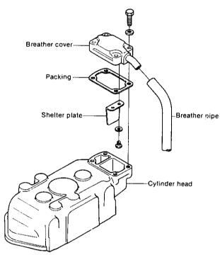
The deflector panel fitted to the breather lid enters the air chamber, and forces air circulation.
