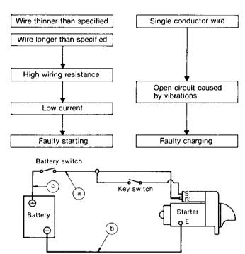
The overall lengths of the wiring between the battery (+) terminal and the starter (B) terminal, and between the battery (-) terminal and the starter (E) terminal should be based on the following table.
