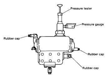
Leakage test using a pressure tester
