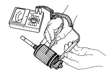
Checking armature windings for insulation faults.
