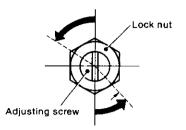
Valve clearance adjusting screw M8 × 1.25 (0.3149 × 0.0492)
